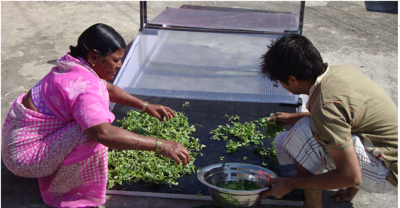
S4S Technologies' microentrepreneur partners dehydrate agricultural produce with a solar conduction dryer
